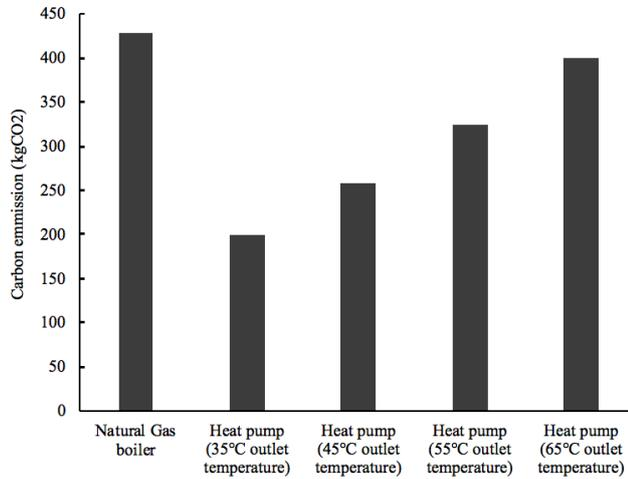
**Fig. 8.** Six-year average CO<sub>2</sub> equivalent for heating using five different heating systems.
