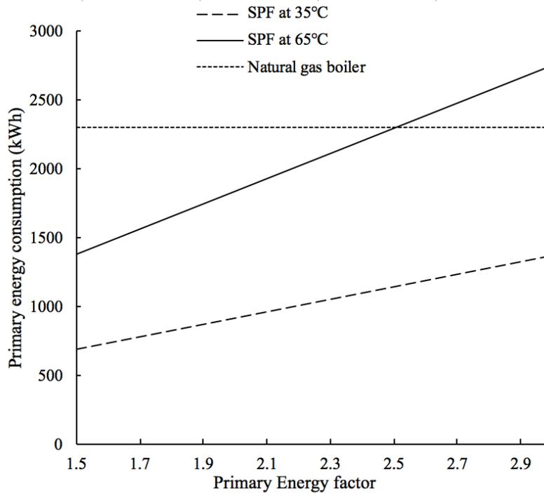
**Fig. 7.** Change in primary energy required for heating consumption with respect to the primary energy factor.
