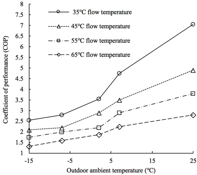
**Fig. 3.** COP vs Ambient temperature for a typical 9kW heat pump tested to in accordance to EN14511-2 [7].
