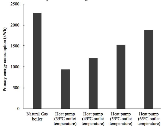
**Fig. 6.** Six-year average primary energy consumption for heating using five different heating systems.
