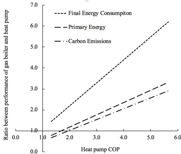
**Fig. 9.** Ratio between the performance of a heat pump and gas boiler for three different metrics, final energy consumption, primary energy and carbon emissions.
