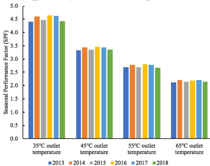
**Fig. 5.** Average COPs at four different outlet temperatures for six different years.
