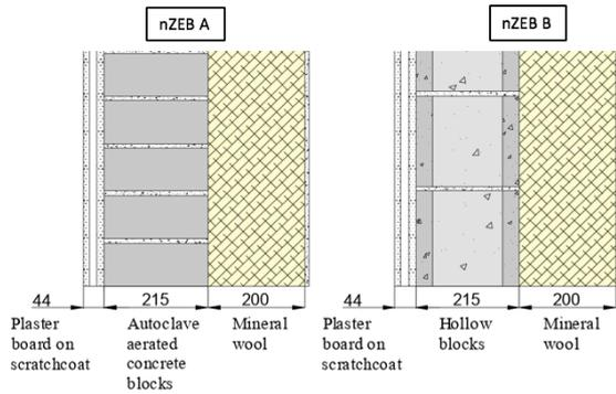
Figure 3. Wall sections for the two nZEB walls
