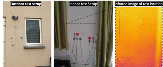
Figure 2. In-situ U-value measurement set-up for example wall.
