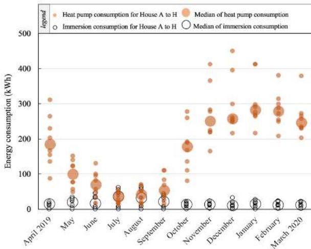
Figure 6. Breakdown of space heating and immersion consumption of the 8 homes.
