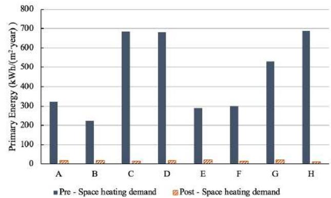
Figure 4. Primary energy requirement for space heating before and after retrofit.
