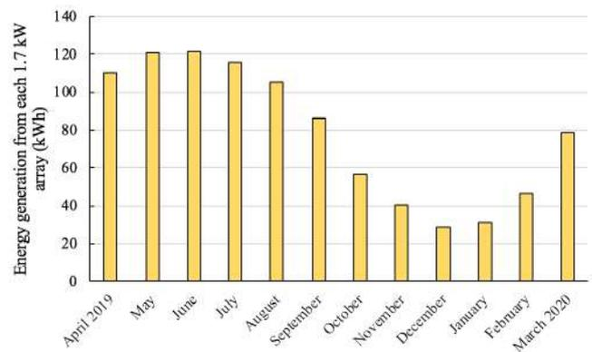
Figure 5. Monthly average energy contribution from each 1.7kW solar array – as per PVGIS calculations [15].
