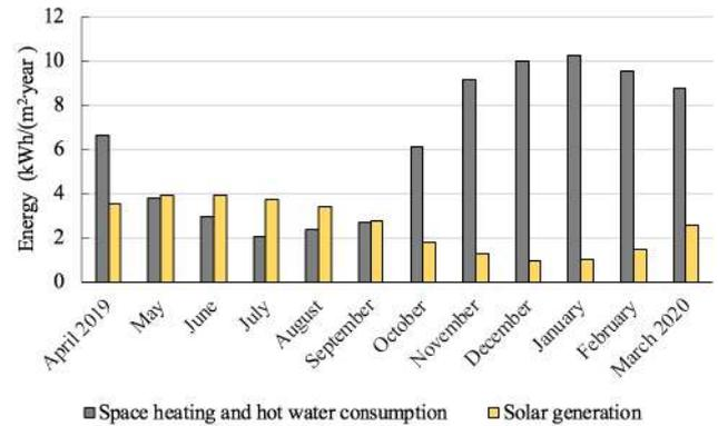
Figure 8. Average combined space heating and hot water consumption per m<sup>2</sup> and estimated solar contribution from each 1.7 kW PV array.
