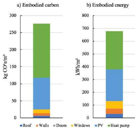
Figure 10. a) Embodied carbon (kgCO<sub>2</sub>e) and b) embodied energy (kWh) per m<sup>2</sup> of building floor area used to complete the upgrade of the 8 homes.
