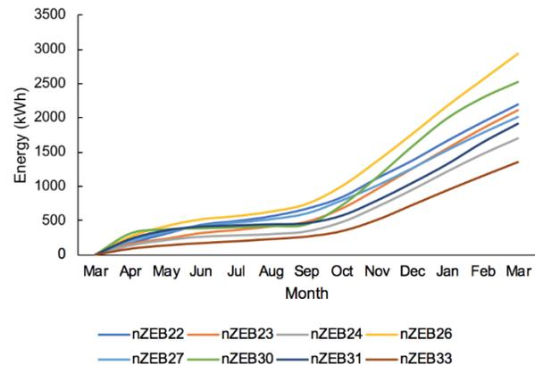
Figure 1. Energy consumption of heat pumps in Irish homes shown as cumulative energy consumption (kWh) against time.
